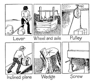
Draw the six simple machines and explain how they are being used in each picture.
