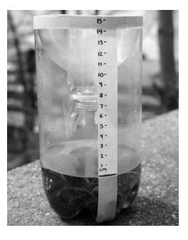
disturbed. There shouldn't be anything hanging over the gauge that could either block any rain or make extra raindrops drip into the bottle (like a tree or a power line or the edge of a roof).
