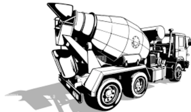
The concrete is mixing while the truck is driving along.
