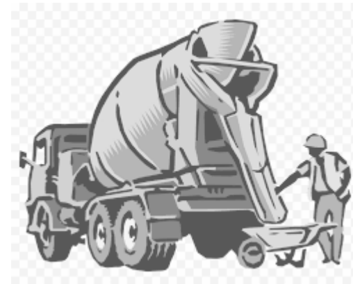
A mixer truck has a tank, mixing blades, a funnel and a chute.
