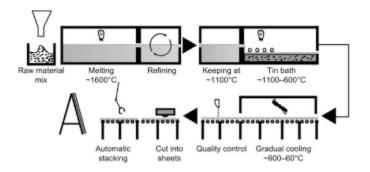
heating→ floating→ cooling→ washing→ cutting→ stacking→ transporting
